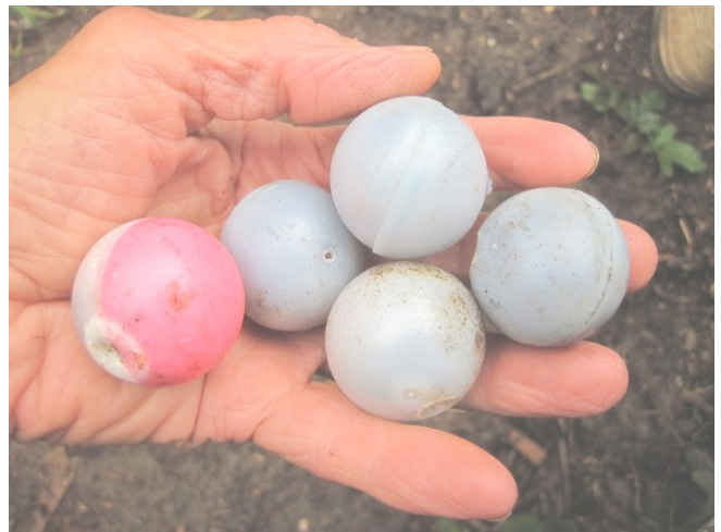
IGNITION BALLS DROPPED BY HELICOPTER
